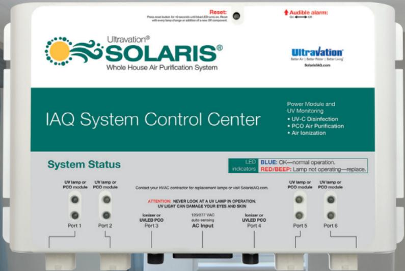
**Reset:** Press and hold for 10 seconds until the LED turns off. Reset with every lamp change or addition of a new UV component.
